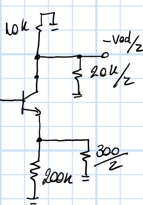
$$\left\{ \begin{array}{l} r_{ea} = \frac{V_T}{0.15mA} = 50\Omega \\ r_o = \frac{VA}{I_C} = 202k\Omega \end{array} \right.$$
