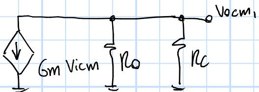
$$\frac{V_{ocm_1}}{V_{icm}} = -G_m \cdot (R_o // R_C)$$
