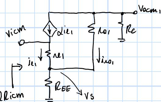
$$\Rightarrow Sabemos \ que \ 2R_{icm} = \frac{V_{icm}}{i_{b2}} = \frac{(\beta+1)V_{icm}}{i_{e1}}$$
