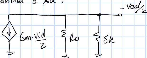
$$\text{onole } G_m \cong \frac{1}{r_{\text{in}} + 200k/\text{V}} = 5 \text{ mA/V}$$
