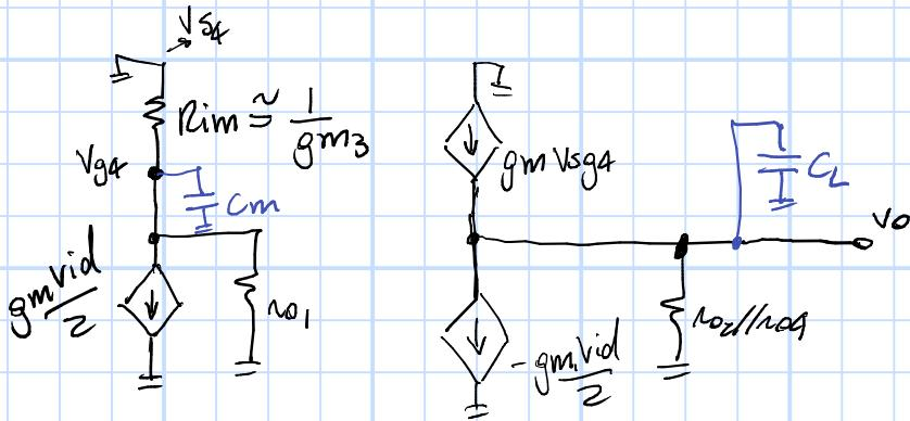
$$V_{g4} = -\frac{gm \cdot vid}{Z} \cdot \left( \underbrace{R_{1m} \parallel r_{01}}_{\sim 1/gm_3} \parallel \frac{1}{5cm} \right)$$
